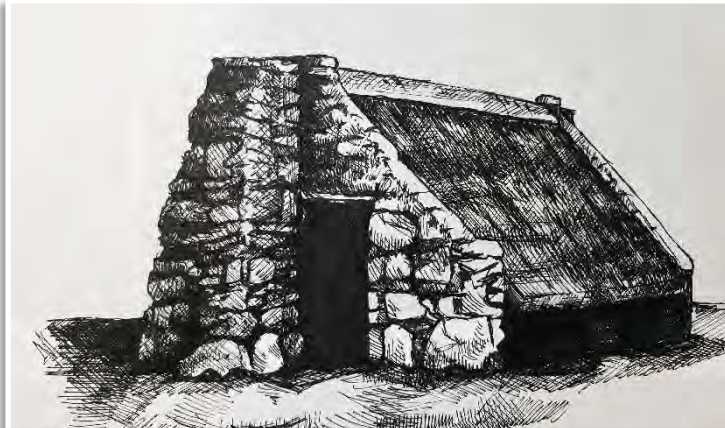
Later Kapstijl house with A-framed stone wall and thatch roof. Image: H. Fivaz
