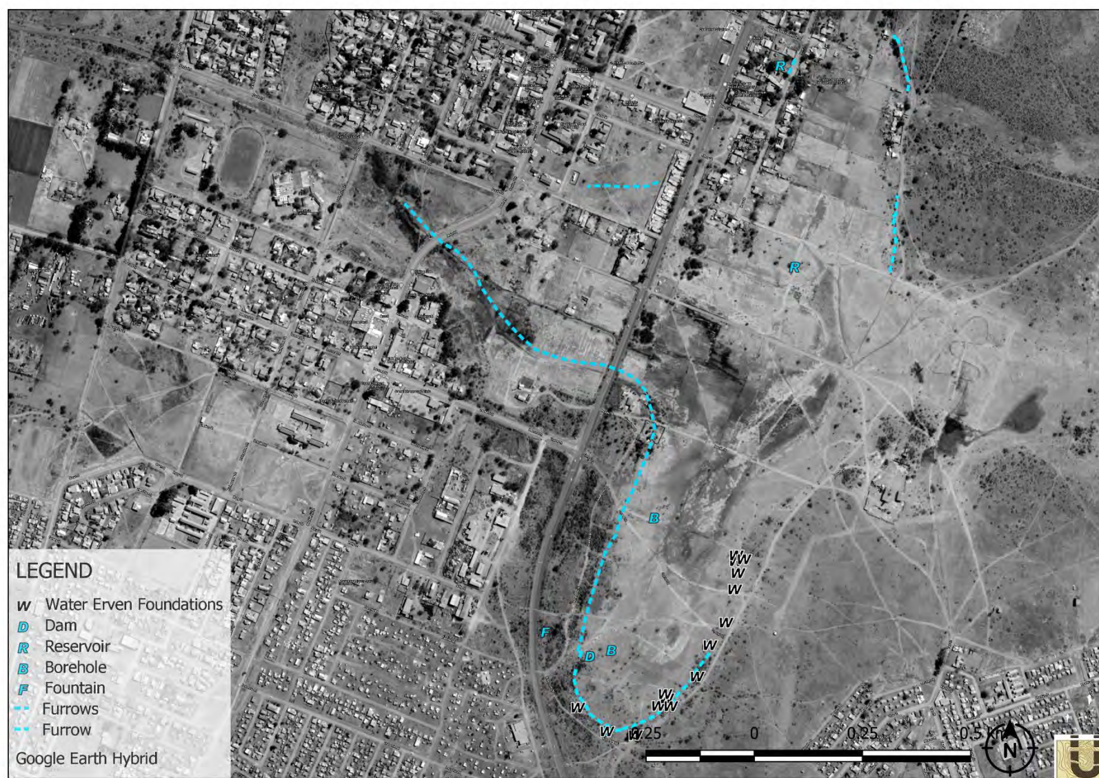
Figure 14 The water furrows and water storage, as part of irrigation scheme. Image: UBIQUE Heritage Consultants
