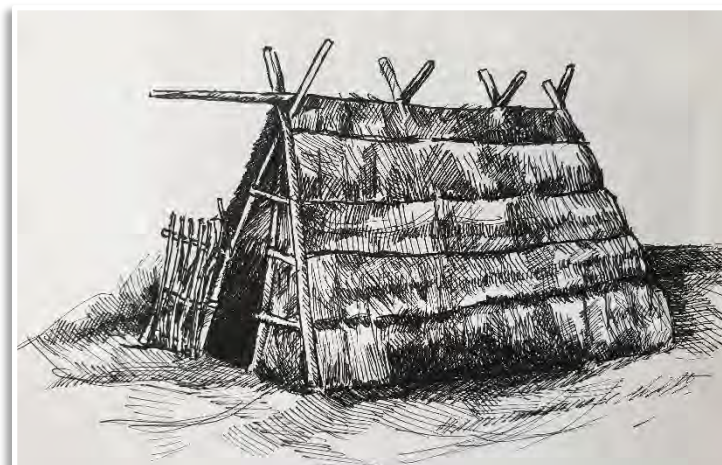
Early Kapstijl house made of thatch, reeds and wooden A-frame. Image: H. Fivaz
